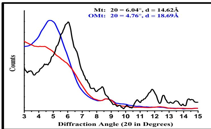
Fig. 5: XRD patterns of Mt, OMt and OMt-MTZ complex
