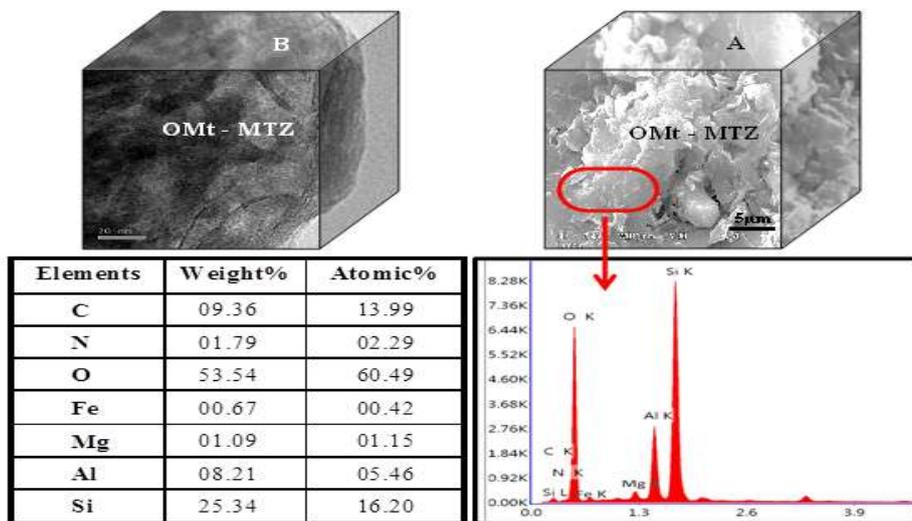
Fig. 7: SEM (A) and TEM (B) image of OMt-MTZ complex with EDX data
