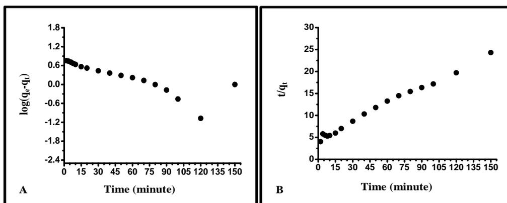
Fig. 4: Kinetic model for the adsorption of MTZ on OMt: (A) Pseudo-first order (B) Pseudo-second order
