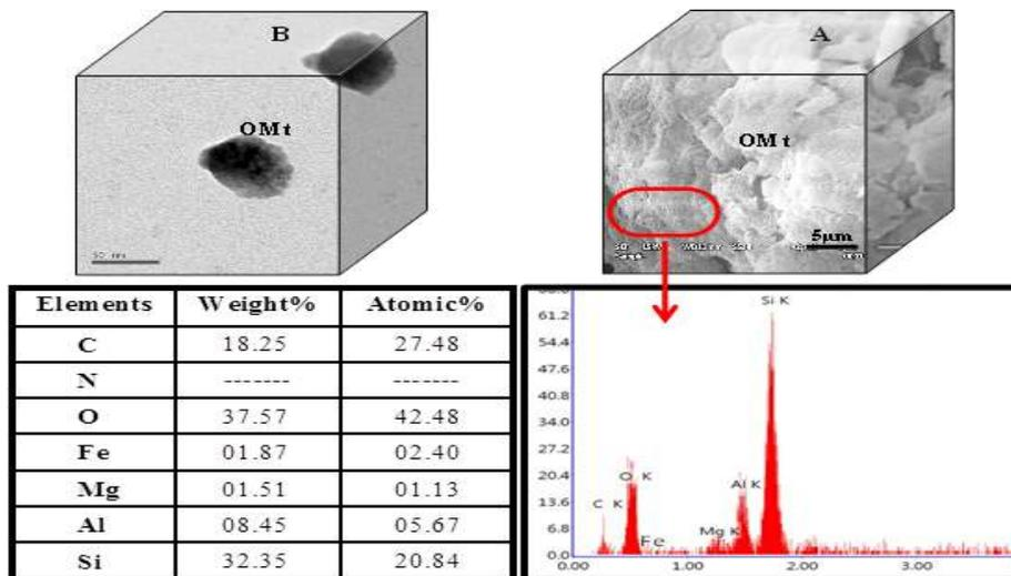
Fig. 6: SEM (A) and TEM (B) image of OMt
