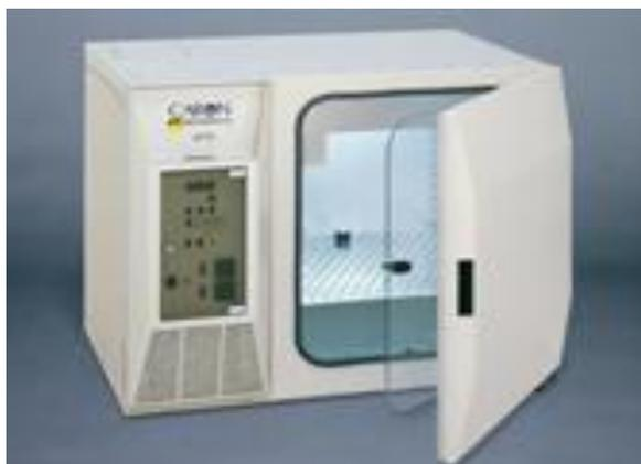
**Fig.1: Photostability Chamber meets requirements of ICH Q1B**
