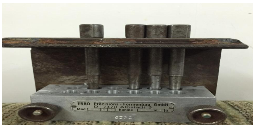
Figure (2): A modified mold (2gm) for preparation of hollow-type suppositories.
