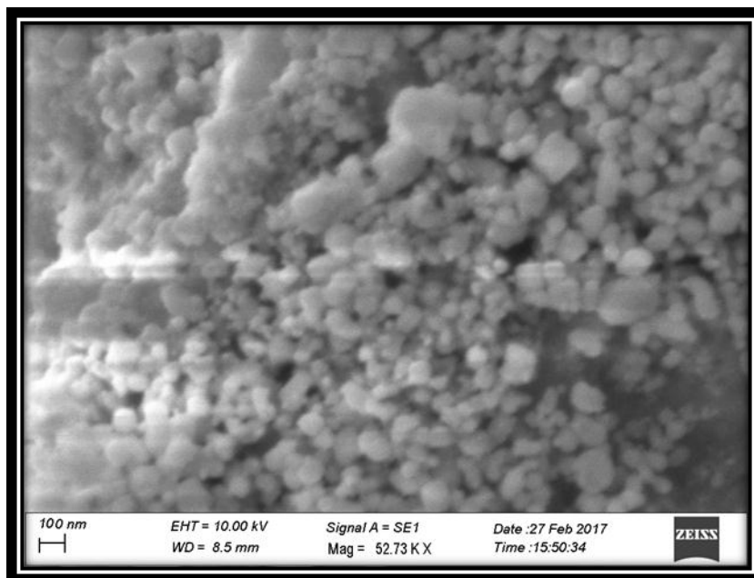
Figure. 3: The SEM image showed the high density silver nanoparticles synthesised in Gymnema sylvestre .
