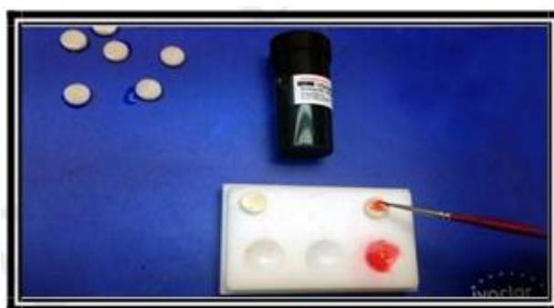
Fig. (2): applying HF acid on the surface of the sample.
