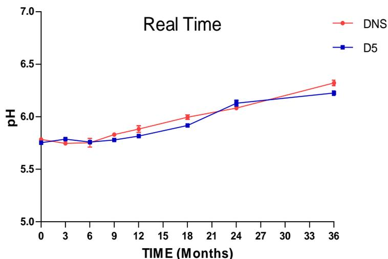
**Figure 1: pH of DNS and D5 in real time study, the initial pH of DNS and D5 were 5.79 and 5.75 respectively. It was observed that pH was raised gradually with increment of days.**
