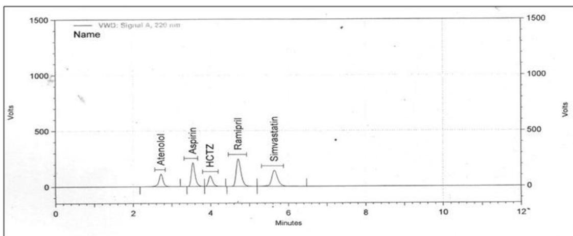
**Figure 1:** A representative chromatogram of mixed drug standard for system suitability.
