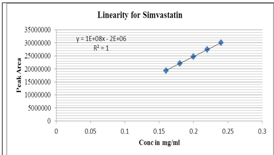
**Figure 3: Calibration curves for drugs.**
