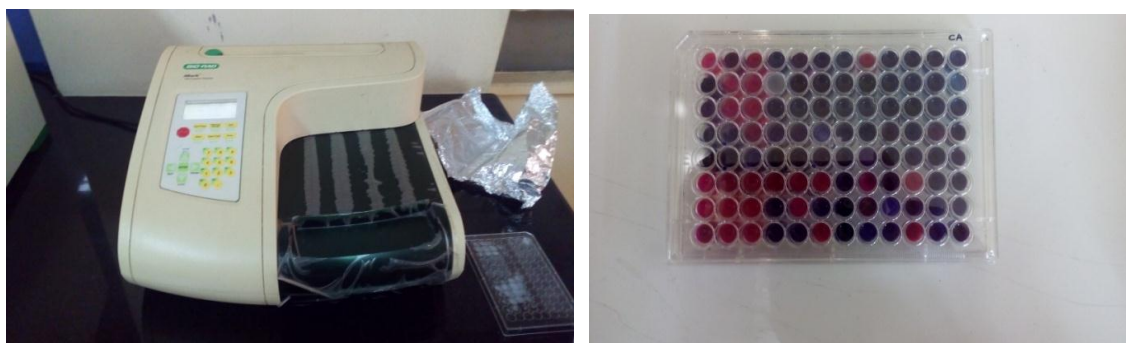
Figure 4: Images showing ELISA READER and 96 well plate used in REMA Assay of anti microbial screening method against S.mutans
