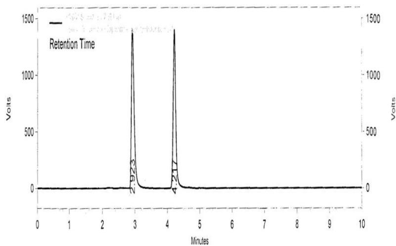
**Figure 7: Chromatogram of alkaline degradation.**
