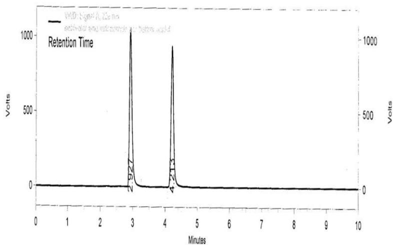
**Figure 8: Chromatogram of peroxide degradation.**
