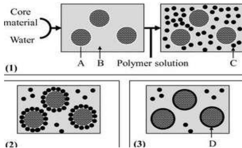
**Figure 5: Scheme of microencapsulation process by coacervation.**
