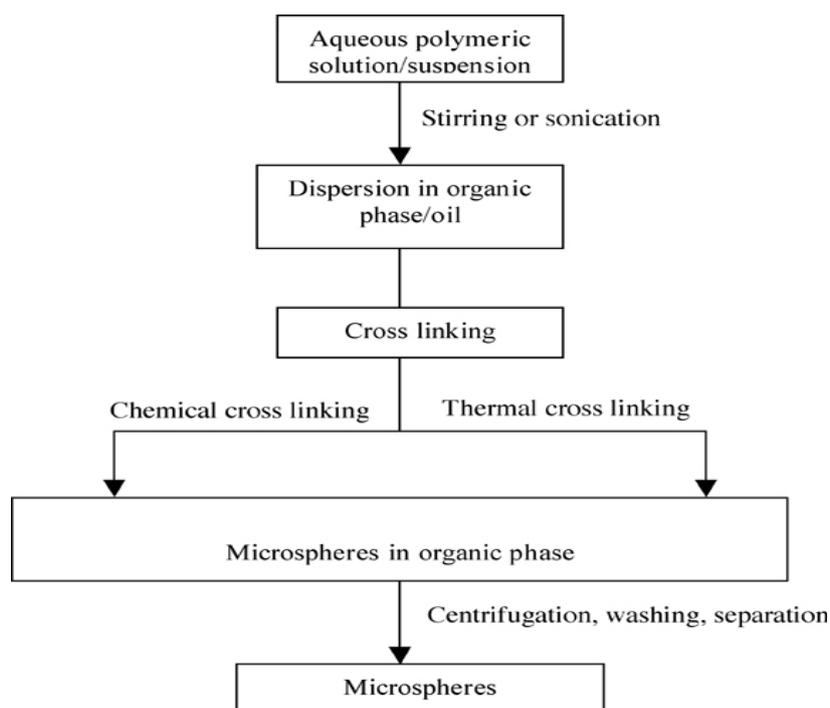
Fig. (4): Schematic representation of simple emulsion method.
