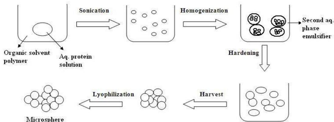
**Figure 6: Solvent evaporation method for preparation of microspheres.**
