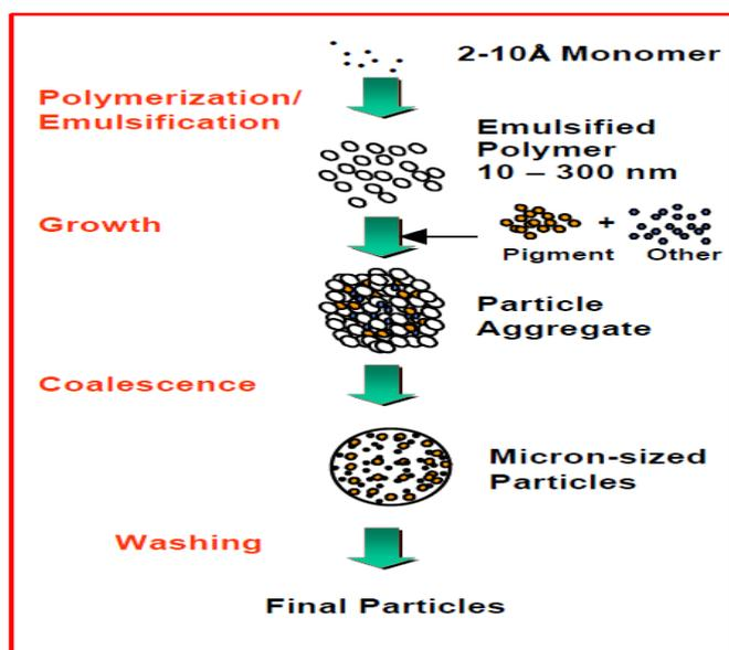
Figure 8:-multiple emulsion polymerization technique.
