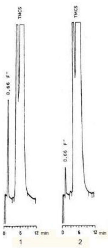
**Fig. 1: Fluorine content in fluorinated material before and after thermal treatment.**
