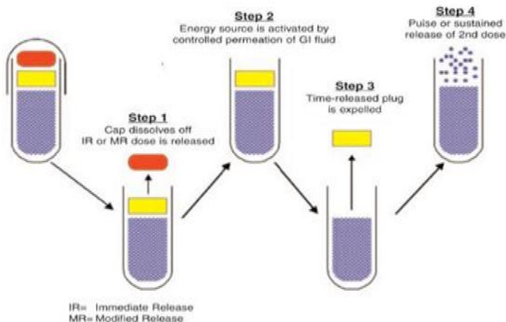
**Figure 4: Drug release mechanism from PORT system.**
