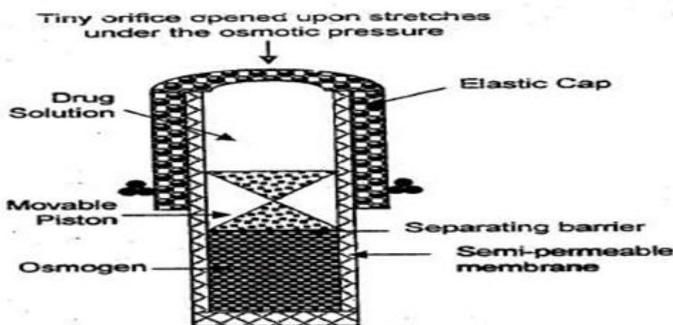
**Figure 5: System based on expandable orifice.**
