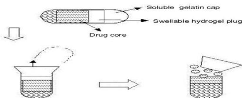
**Figure 3: Design of Pulsincap system.**
