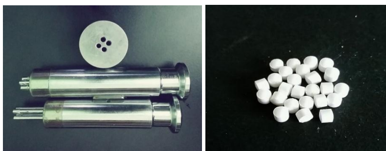
“Fig. 1” Multi-tip punch (4mm) die and core tablets.
