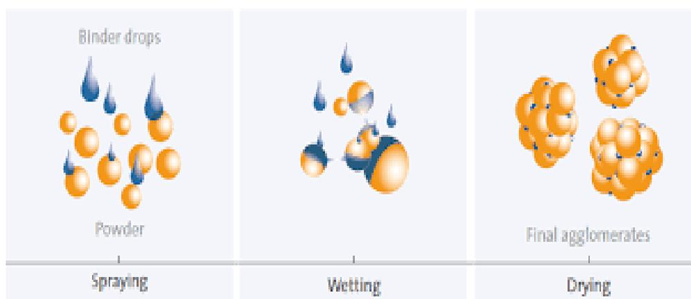
Figure No. 2 Process principle of fluid bed dryer.
