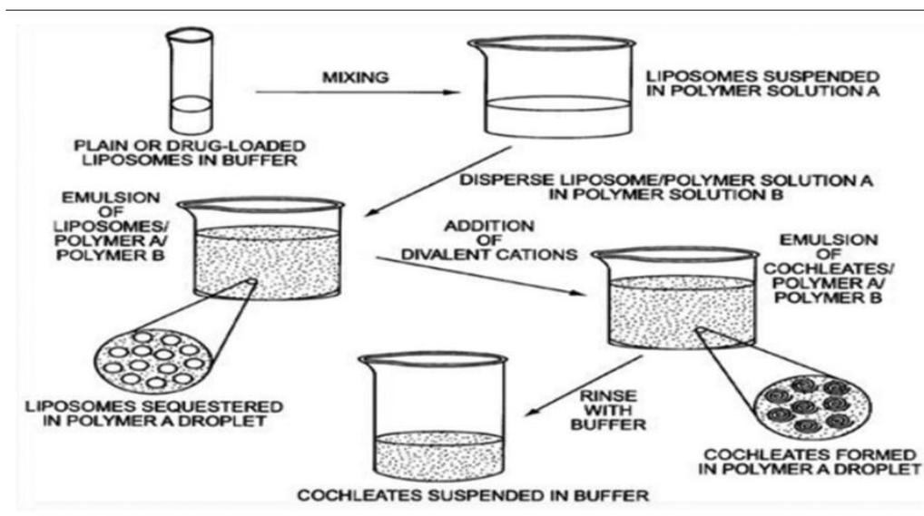
Fig. 5: Preparation of Nanocochleate by Hydrogel method.<sup>[2,33]</sup>
