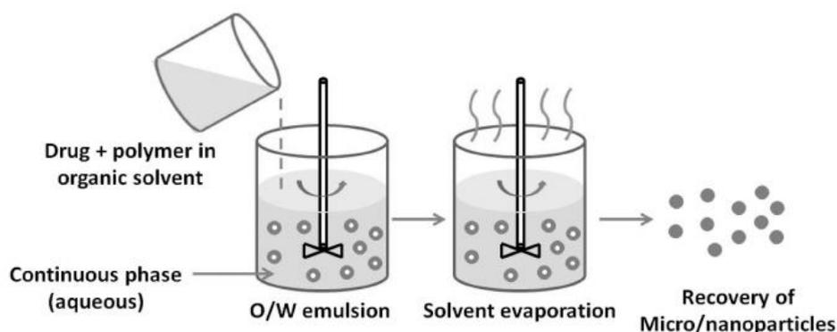
**Figure 1: Emulsion Solvent Evaporation Method.**
