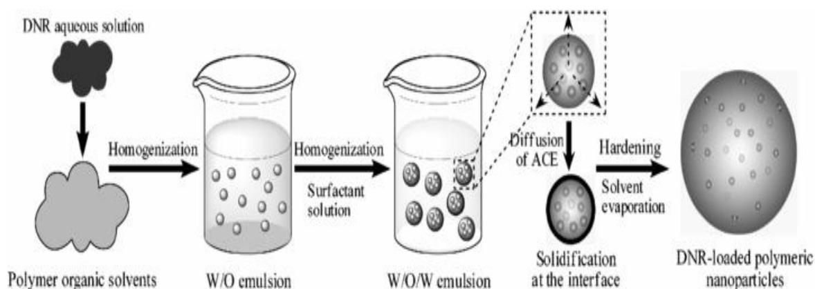
**Figure 2: Double Emulsion and Evaporation Method.**
