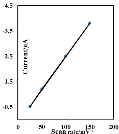
**Fig. Effect of scan rate on ZPLN at pH 6.0 in phosphate buffer solution at Concentration:  $2.25 \times 10^{-7} \text{M}$  at different scan rates: 50mV/s to 200mV/s.**
