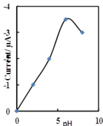
**Fig. The plot of the current Vs pH of zopiclone in PB solution, Concentration:  $2.55 \times 10^{-7}$  M at glassy carbon electrode at different pH values (pH 2.0-8.0).**
