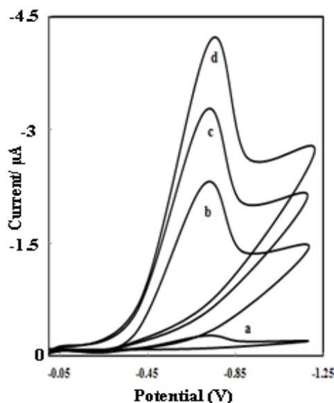
**Fig. Cyclic voltammograms of  $2.25 \times 10^{-7}$  M zopiclone, at pH 6.0 of phosphate buffer at glassy carbon electrode at different scan rates (50 mV/s-200 mV/s).**
