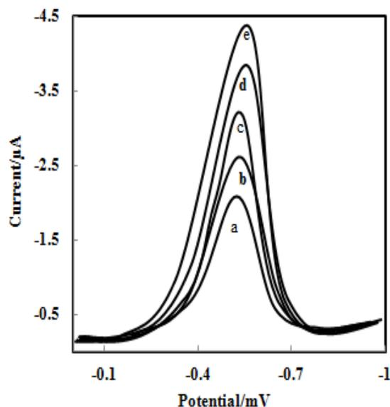
**Fig. Typical DPV of zopiclone in phosphate buffer solution at pH 6.0, Concentration:  $2.25 \times 10^{-7} \text{M}$  to  $6.42 \times 10^{-4} \text{M}$  at GCE.**
