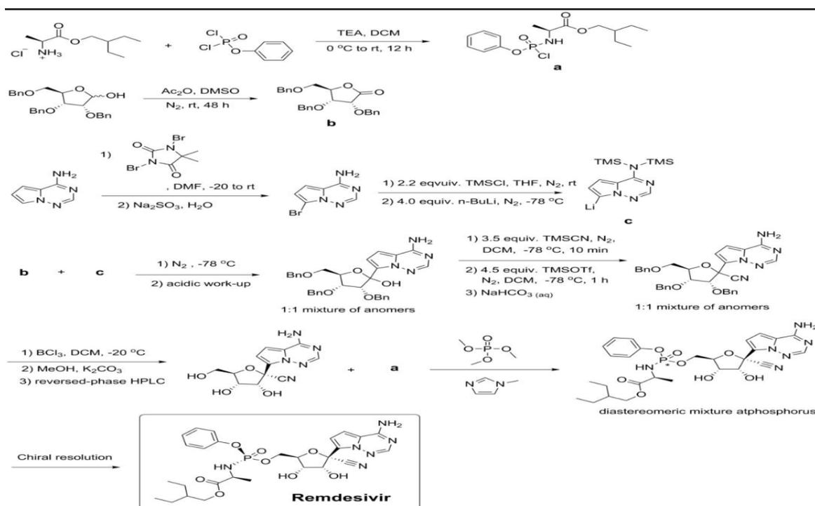
**Fig. 3:** synthesis of remdesivir invented by byoung kwan chun et.al. from gilead sciences.
