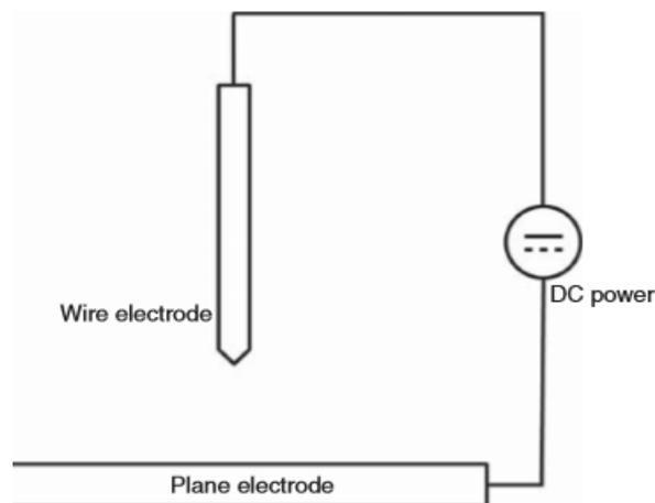
**Fig. 4: Corona Discharge (Schematic Representation).**
