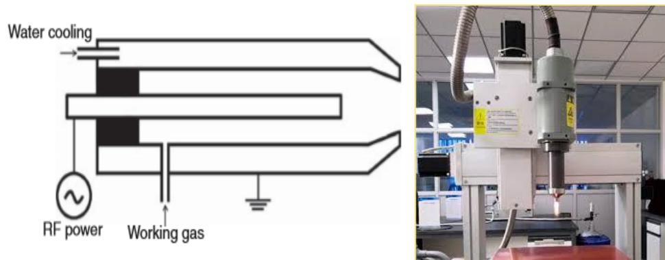
**Fig. 3: Schematic Diagram of Cold Plasma Jet.**
