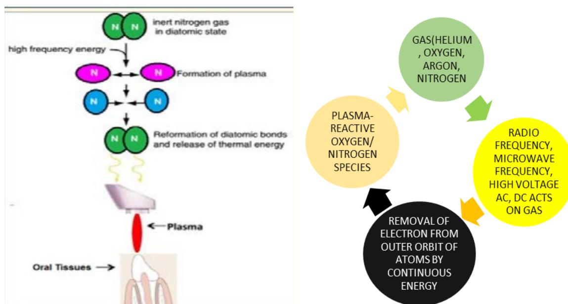
**Fig 1: Shows Nitrogen gas being acted upon by high frequency energy to cause dissociation of gas by stripping of electrons and generation of plasma.**
