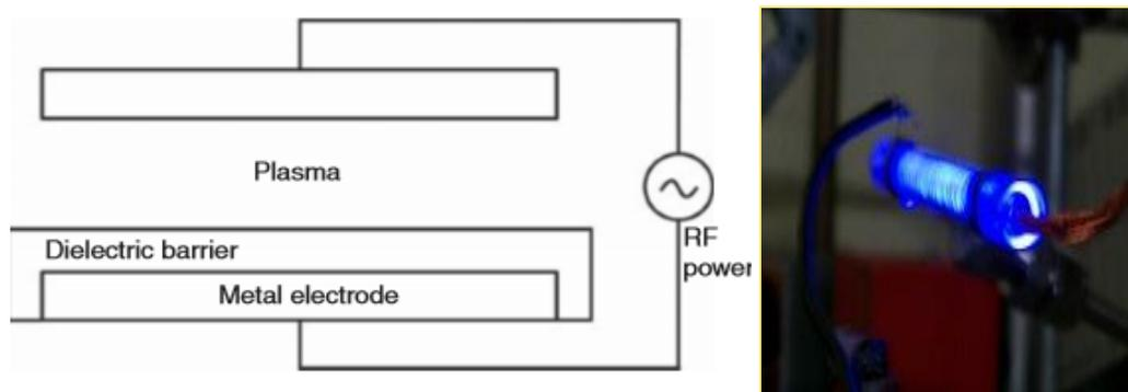
**Fig. 2: Schematic Diagram of a Dielectric Barrier Discharge.**
