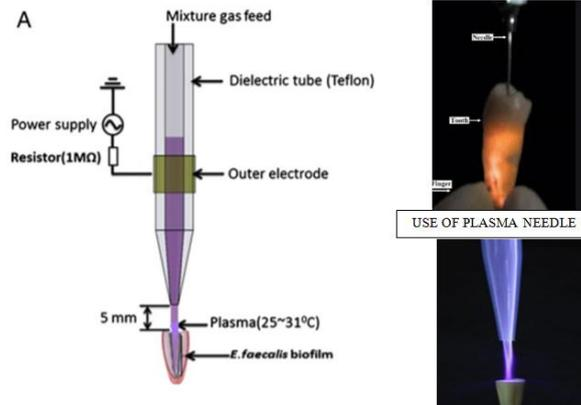
**Fig 7: Schematic diagram of mechanism of action of plasma needle- distance between tip of nozzle and tooth sample should be greater than 5mm.**
