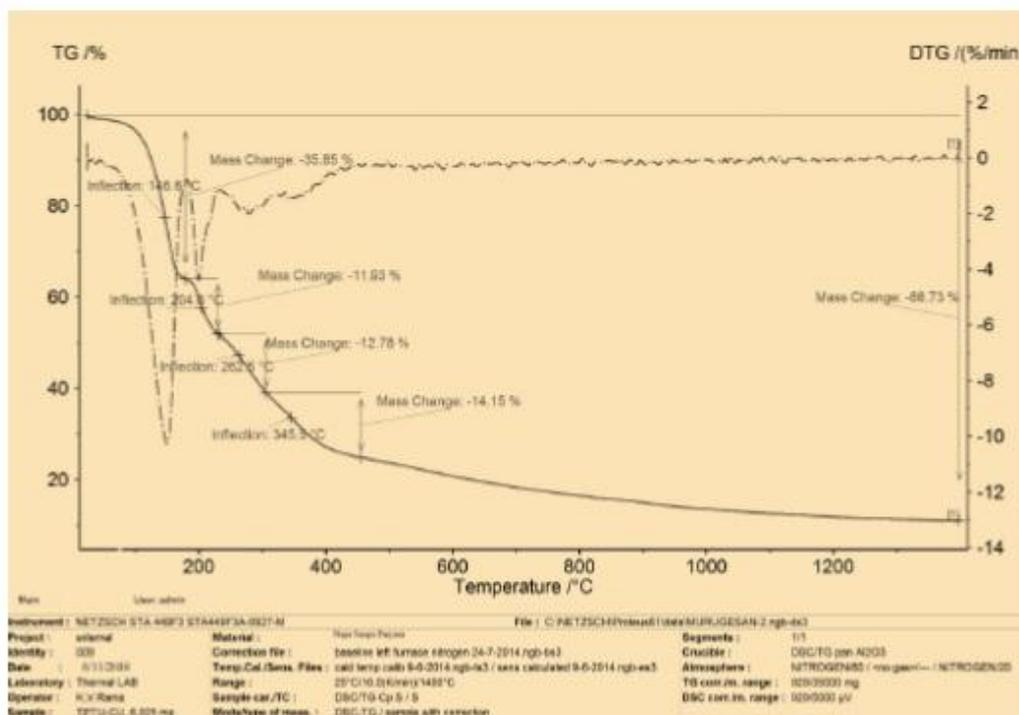
**Figure 2: Thermo Gravimetric Analysis of Naaga Sangu Parpam.**
