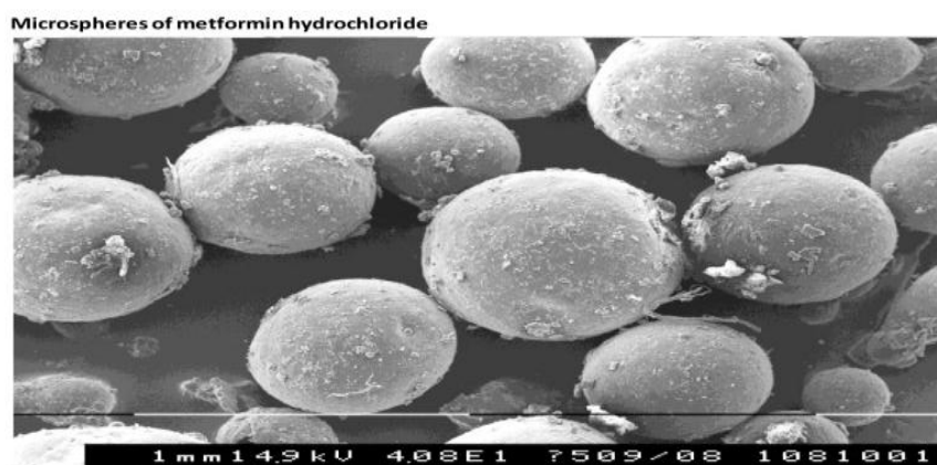
Figure 4: SEM photograph of metformin hydrochloride floating microspheres
