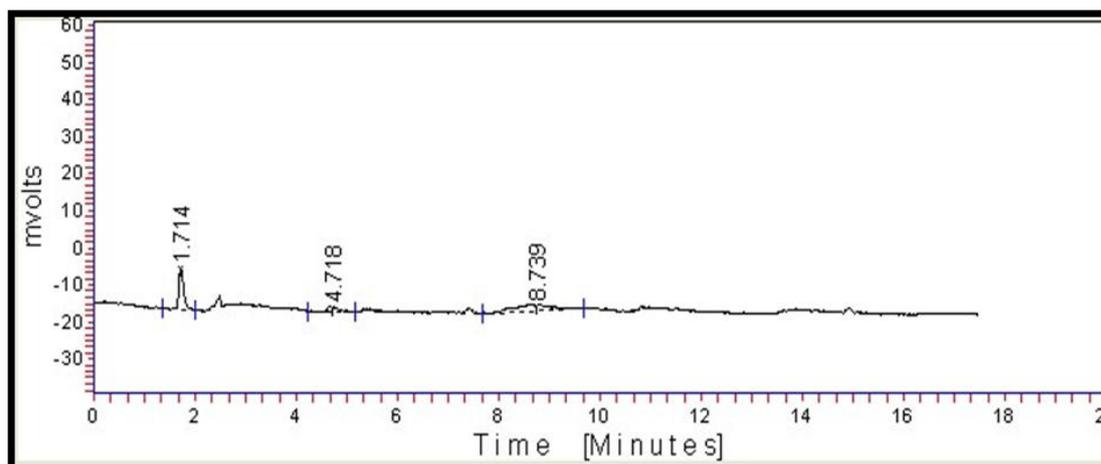
**Figure 3: Chromatogram of sample extract G-2 for quantitative estimation of malathion in ladyfinger samples washed with vinegar solution at 230 nm.**
