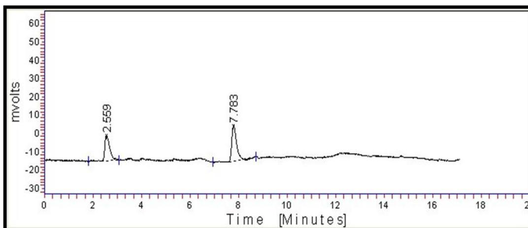
**Figure 3: Chromatogram of sample extract G-2 for quantitative estimation of malathion in ladyfinger samples washed with rock salt solution at 230 nm.**
