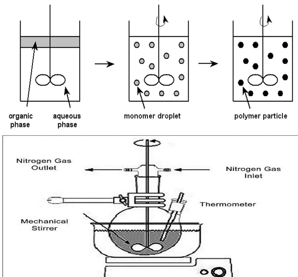
Figure 2: Liquid-liquid suspension polymerization.
