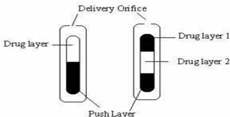
Fig. 1: Bi-layer and tri-layer OROS Push pull technology.
