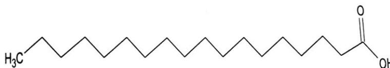
**Structure of Stearic acid**
