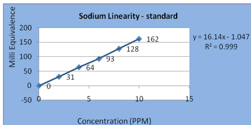
**Fig. 4: Linearity of Sodium Standard.**
